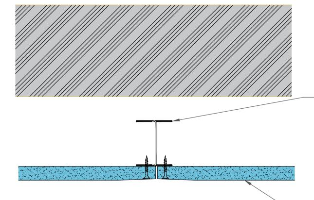
SPEEDLINE 50mm 'I' Studs at 600mm Ctrs
